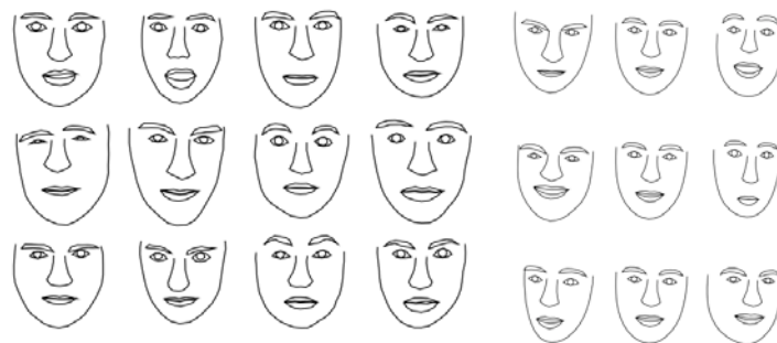
Figure 17 - Left: shapes instances from the training set. Right: shapes resulting when varying the first 3 modes in the model (from Cootes et al 1995)
