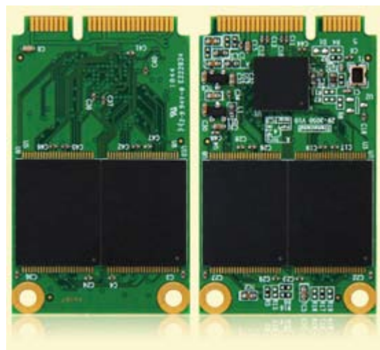
Figure 3: Solid State Disc with the newest mSATA interface [9]
